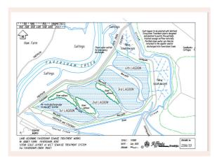
Our proposal to divert the outfall from the Faversham sewage works into a reed bed system gained a lot of positive support, however further findings have shown some drawbacks, reports Eldon Hinchliffe. Reeds spread very quickly and clog up the system and therefore need to be managed. Traditionally this was done
